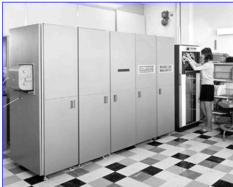
Figure 3. A Stromber-Carlson SC4020 Microfilm recorder at the Atlas Computer Laboratory, Chilton (close to Harwell), in 1967. Similar equipment was installed at AWRE Aldermaston in 1963 and later upgraded to a SC4060.
