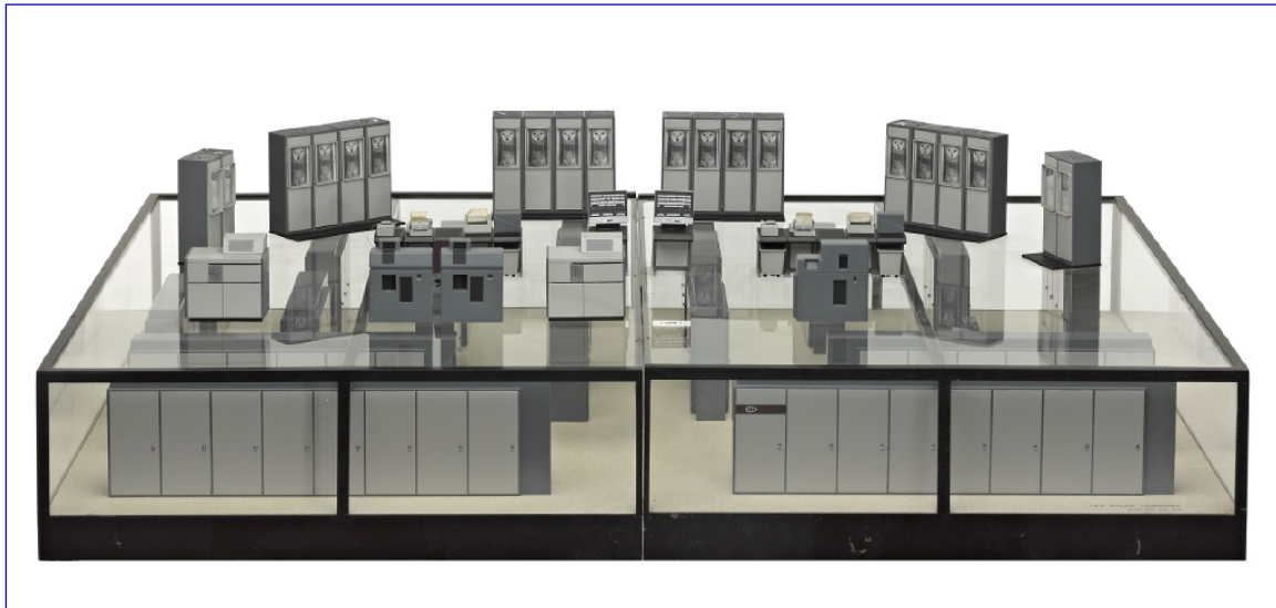
Figure 4. Scale model of a large Atlas installation, showing equipment on two levels. Broadly speaking, the upper floor holds input/output equipment whilst the central processor and memory system occupy the lower floor.
