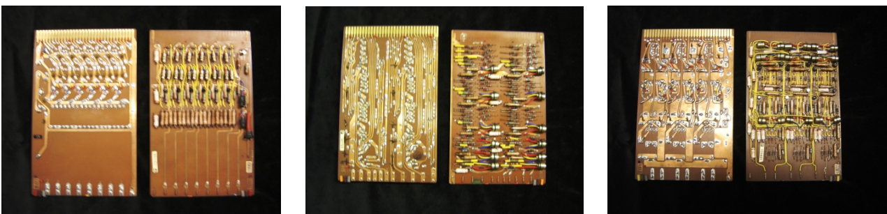
Figure 14. The front and back of three sample Atlas printed-circuit boards from bay 2 of the CPU cabinet. (From left-to-right): type 812 (adder carry), type 813 (adder input) and type 814 (adder output).
