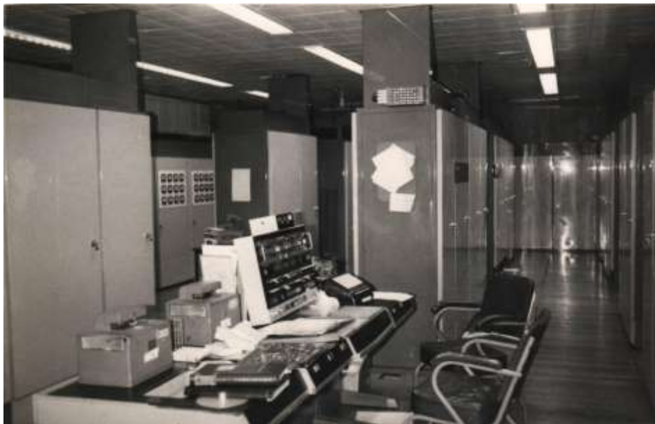
This was the main control desk in the lower room. There was intercommunication between this control desk and the other computer locations. The control desk was donated to the South Kensington Science Museum
