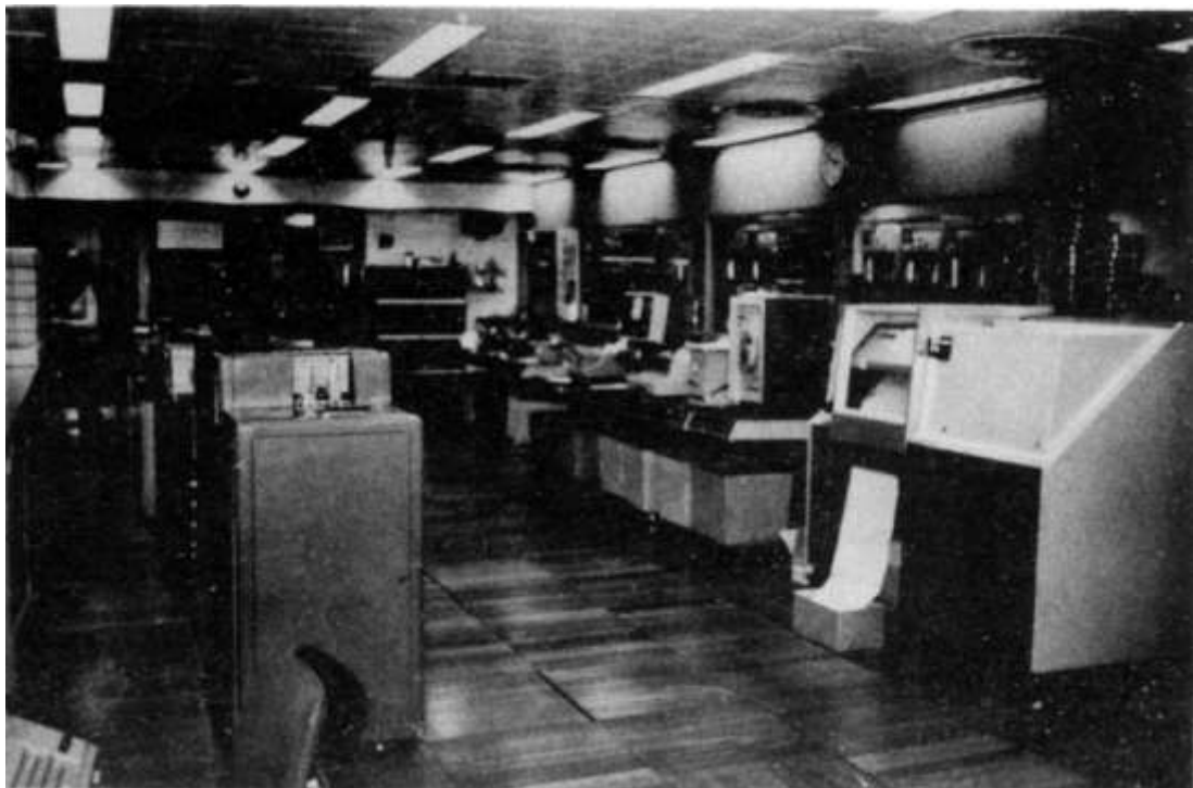
Another view of the computer room with one of the Anelex printers, the magnetic tape in the back ground, and card readers and punches to the left
